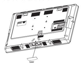
4 Attach the wall-mount bracket with the four screws that come with the wall-mount bracket kit.
